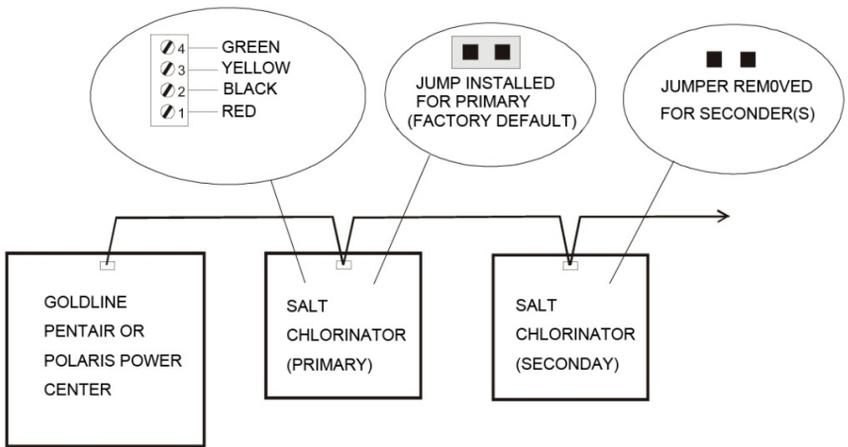
Goldline - Attach wires to proper screw terminals as show below.
