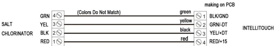
Polaris - Attach wires to proper screw terminals as shown below. Note that screw terminal "1" is marked on the Polaris PCB.
