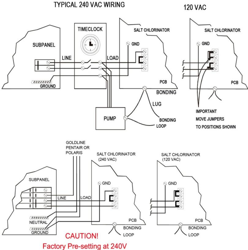
**Note:** Wire the pump directly to the time clock—do not use the salt chlorinator as a junction box.
